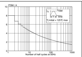
Fig.4. Maximum permissible non-repetitive peak on-state current I<sub>TSM</sub>, versus number of cycles, for sinusoidal currents, f = 50 Hz.
