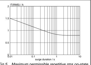
Fig.5. Maximum permissible repetitive rms on-state current  $I_{T(RMS)}$ , versus surge duration, for sinusoidal currents, f = 50 Hz;  $T_{lead} \le 83^{\circ}C$ .
