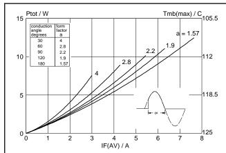
Fig.1. Maximum on-state dissipation,  $P_{\text{tot}}$ , versus average on-state current,  $I_{\text{T(AV)}}$ , where  $a = form \ factor = I_{T(RMS)} / I_{T(AV)}$
