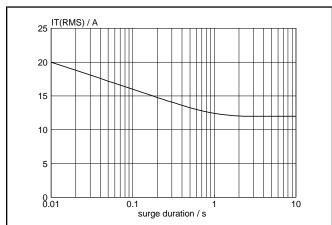
Fig.5. Maximum permissible repetitive rms on-state current  $I_{T(RMS)}$ , versus surge duration, for sinusoidal currents, f = 50 Hz;  $T_{mb} \le 109$ °C.
